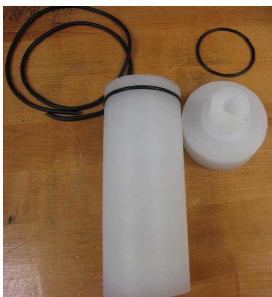
Figure 2.4. Custom-Fabricated Polyethylene Containment Used for B 4 C Irradiations
