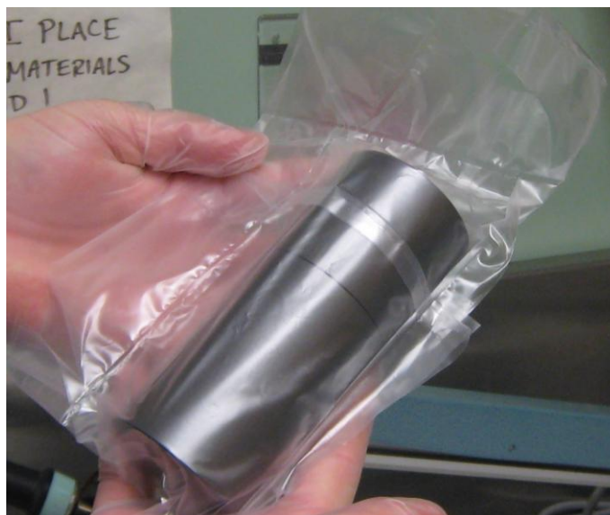
Figure 2.3. B 4 C Shield Sealed in Plastic Before Irradiation
